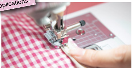
Specialized presser foot can be guided over a concealed zipper - easy enough for anyone to sew neat finishes.
